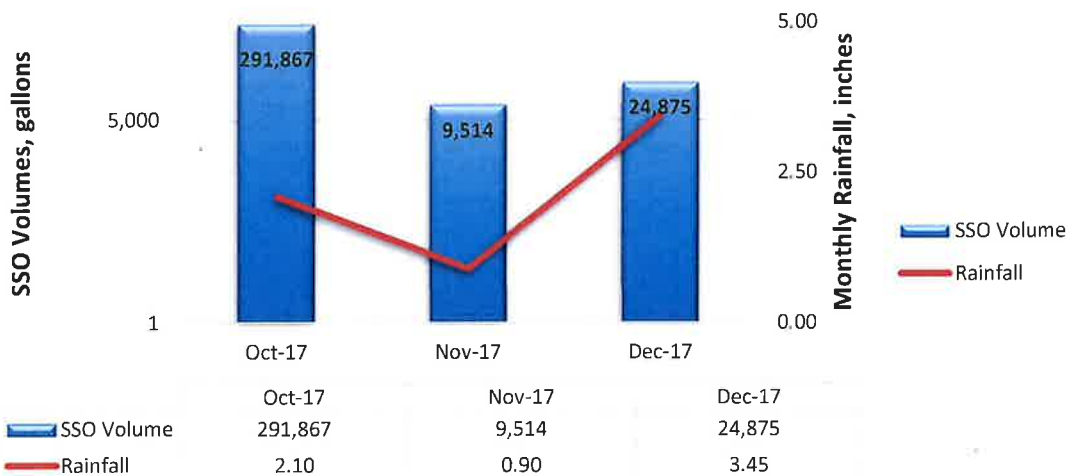
Figure 3: Collection System SSO Volume
