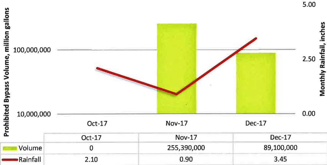
Figure 9: Prohibited Bypass Volume vs. Rainfall
