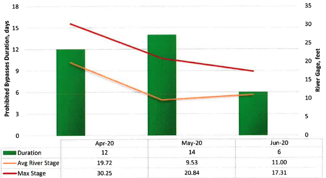
Figure 16: Monthly Prohibited Bypass Duration vs. River Stage
