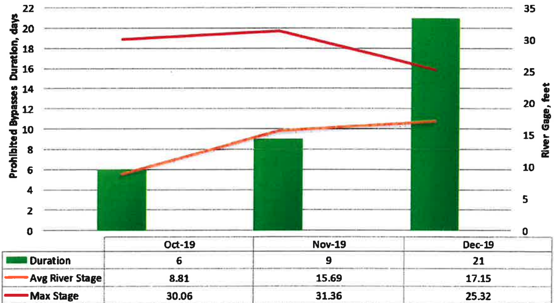
Figure 16: Prohibited Bypass Duration vs. River Stage
